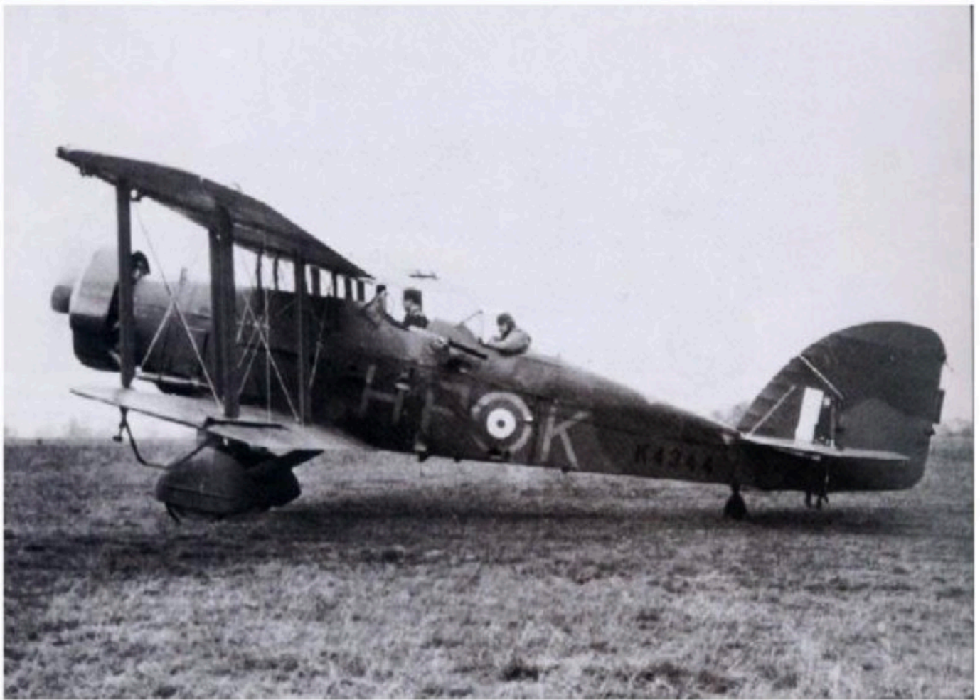
A Westland Wallace showing the cable towing equipment on the fuselage
