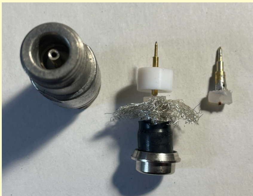
Left to right: female socket, undersize centre pin, correct size centre pin.
